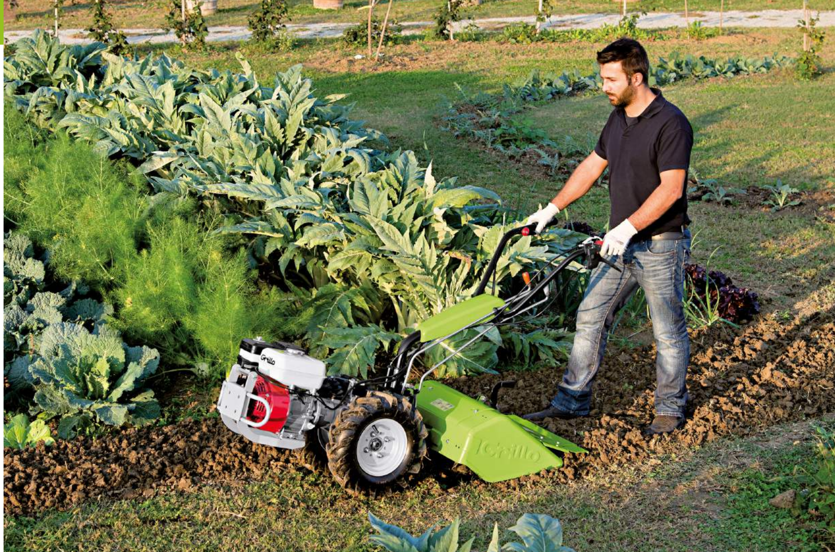
G 84 with furrower behind the rotary tiller.
