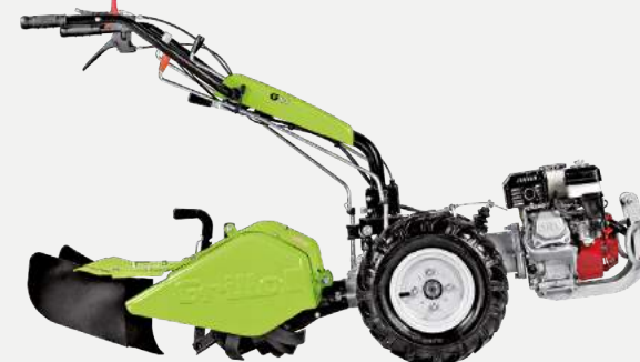
G 84 with furrower behind the rotary tiller.
